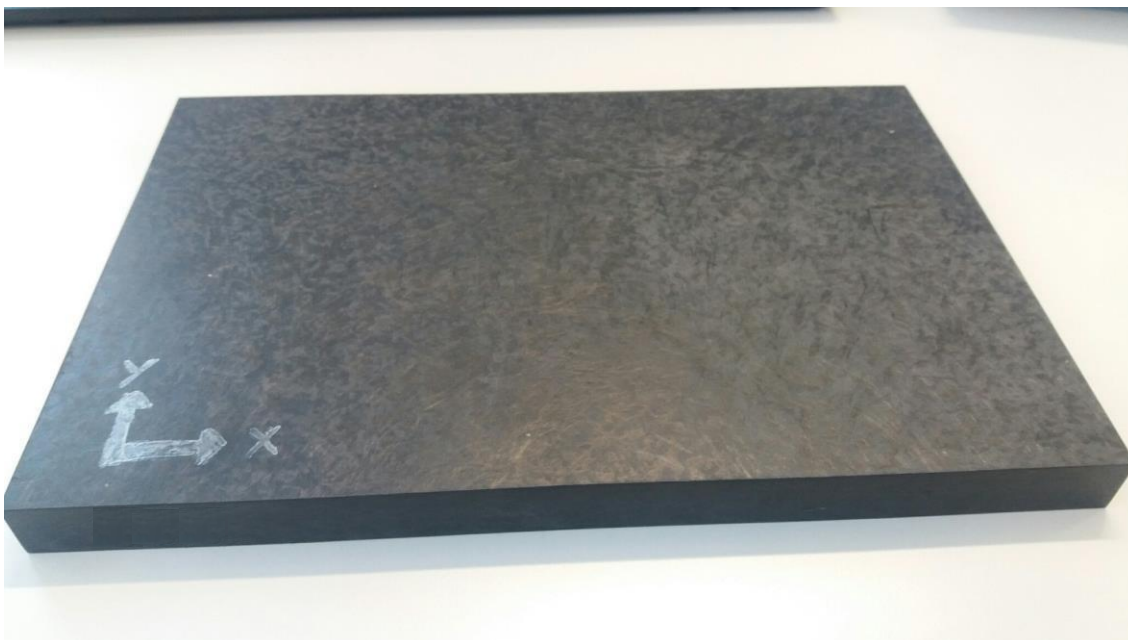
Figure 1. Showing the 360 carbon/nylon block material as received and the X and Y directions used.
